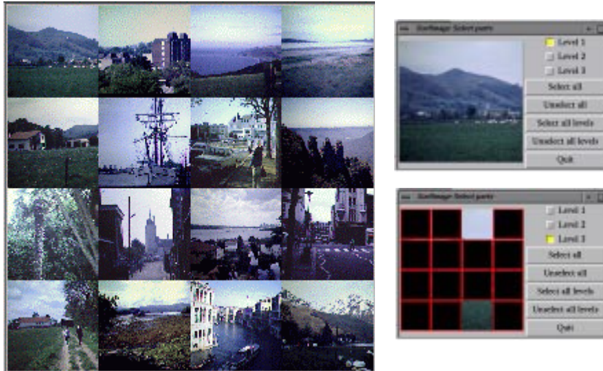
Fig.5 Retrieval of the top left image. Retrieved images are from top left to bottom right in order of best match. Query image at level 1 and partial queries at level 3 are also presented. We search for selections every where in the database images
